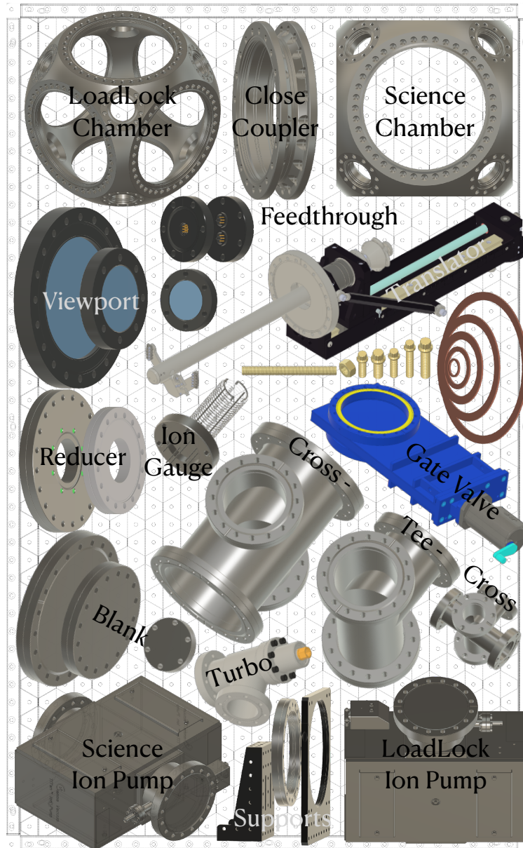
Figure 12.6: A graphical display of components of the loadlock vacuum apparatus.
