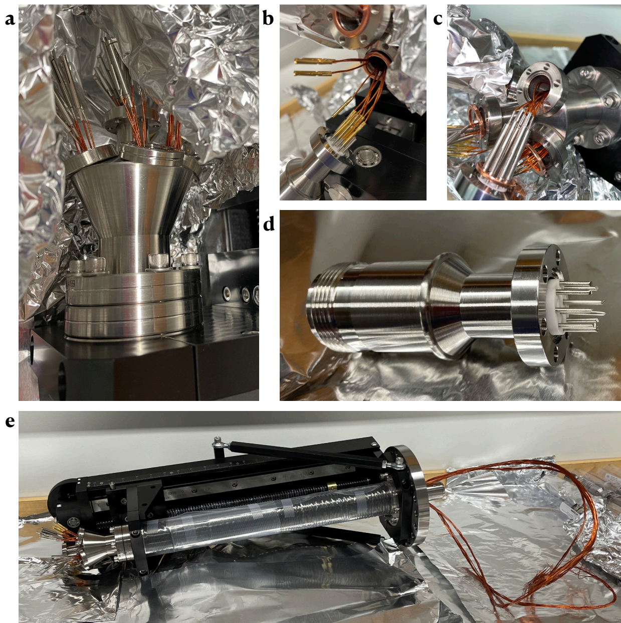
Figure 13.2: Obsolete feedthrough assembly. This feedthrough assembly is now obsolete due to its default setup with the translator, which led to potential electrical shorts between the voltage-carrying pins and the chamber walls, thus consequently replaced. a , the utility feedthrough hat assembly. Failed examples feedthrough connectors with short and long pins in b and c , respectively. d , a feedthrough connector with shortened pins. e , the obsolete feedthrough assembly.
