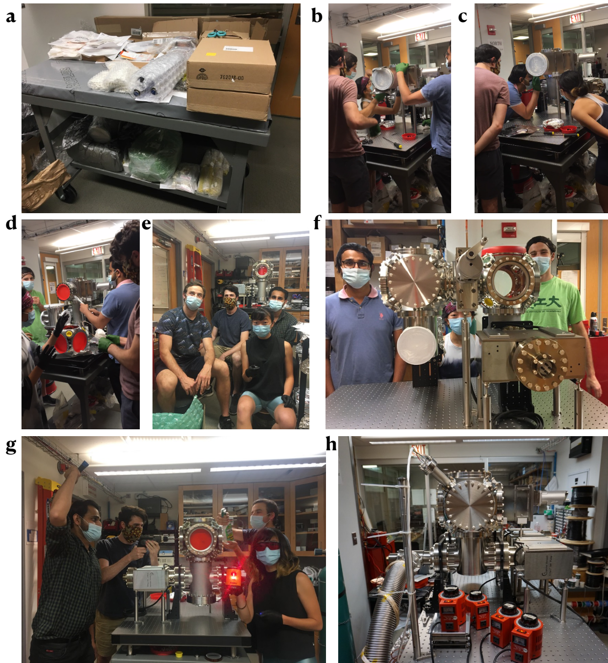
Figure 12.7: Snapshots for Stage I, assembly of the vacuum chamber with the translator temporarily replaced by a blank flange. a , delivery of vacuum system components. b , c , and d , progress during Stage I. e , and f , near-completion of Stage I, lacking one ‘leg’ of the vacuum chamber. g and h , completion of Stage I.
