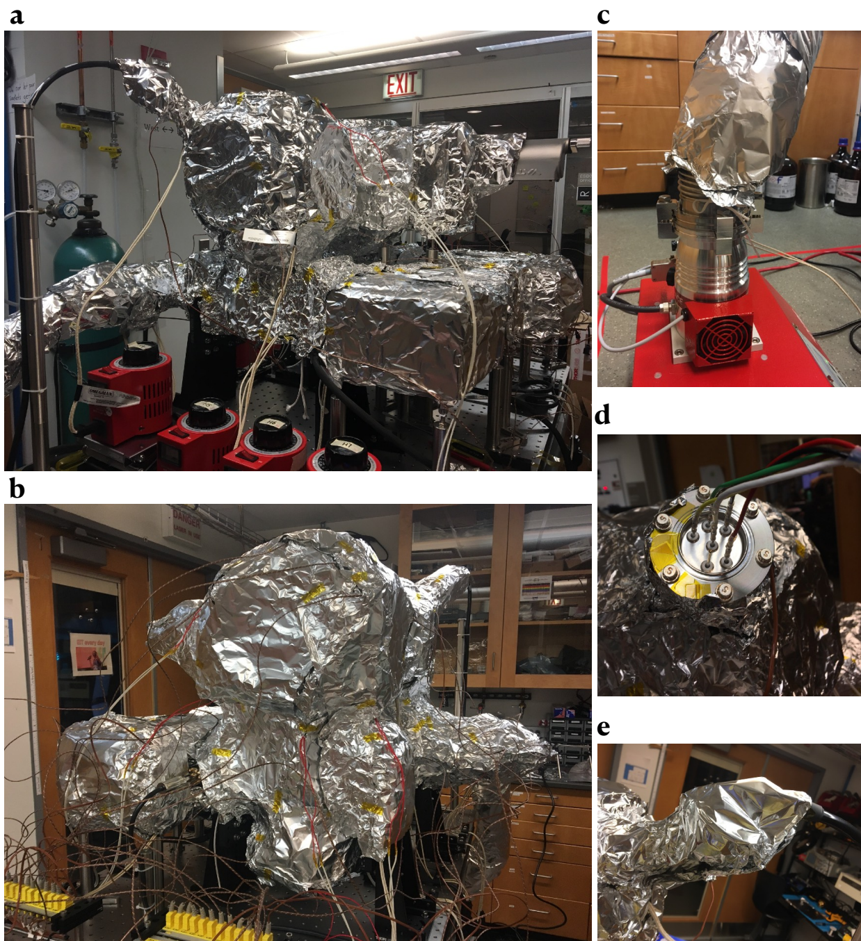
Figure 12.20: Aluminum foil wrapped around the vacuum chamber, lacking the translator, for improved heat retention during bakeout. a , a single from the loadlock chamber's perspective. b , multiple layers from the science chamber's perspective. c , the turbo pump station. d , the ion gauge with exposed pins. e , the ion gauge carefully foiled to prevent electrical shorts.
