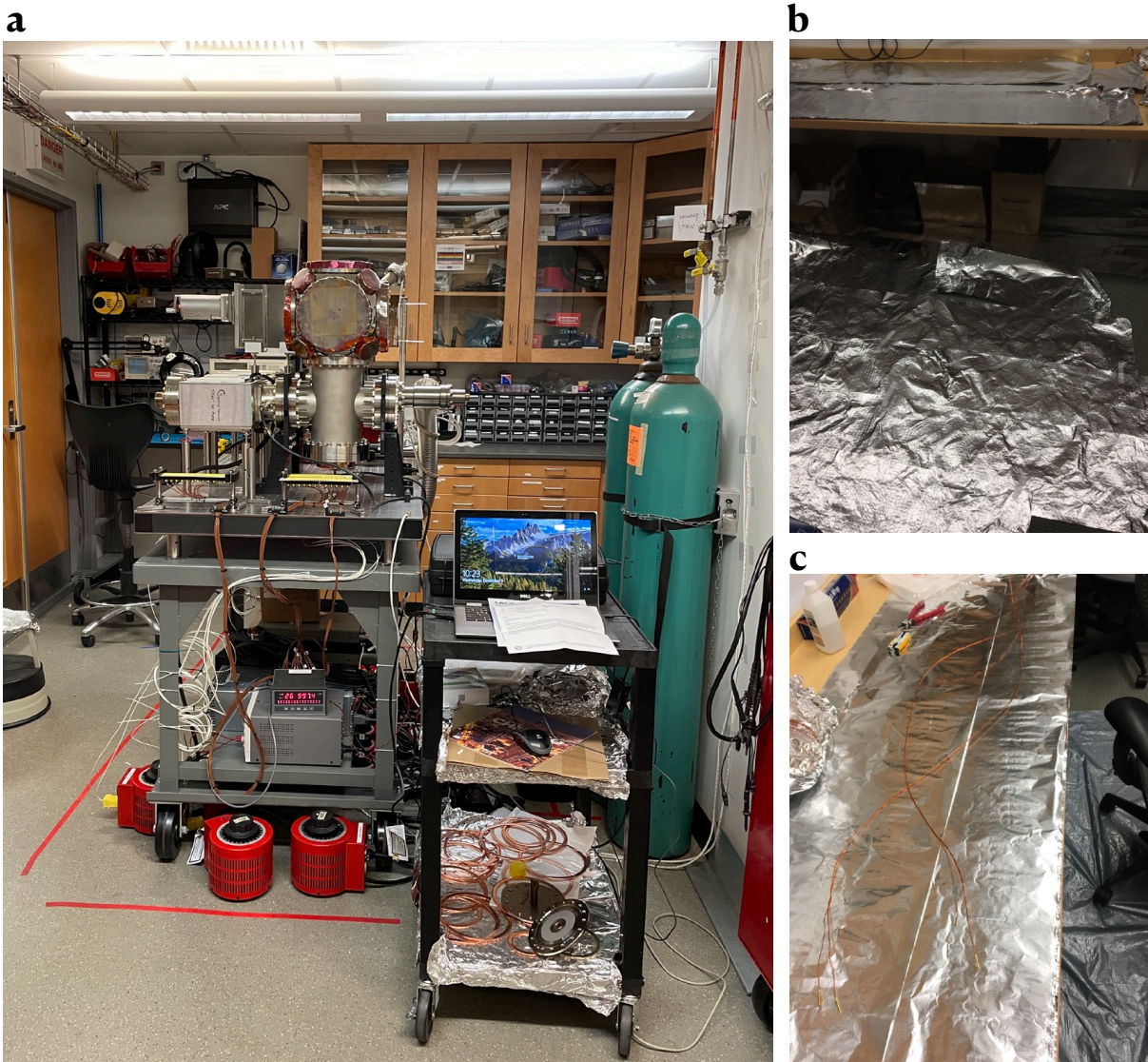
Figure 12.13: The vacuum chamber setup before the neighboring office was renovated to be a lab space. a , the vacuum chamber, lacking the translator, assembled, pumped, and baked on a mobile steel cart situated in the preparation room. Meanwhile, the neighboring office space was transferred into a temporary clean area for meticulous vacuum tasks, such as routing the feedthrough setup through the translator. b and c , to maintain stringent cleanliness standards, the office carpet was shielded with fabric and aluminum foil to prevent any carpet debris from contaminating the air in contact with the vacuum environment. Additionally, layers of aluminum foil were applied to the office tables to ensure cleanliness for direct contact with vacuum components.
